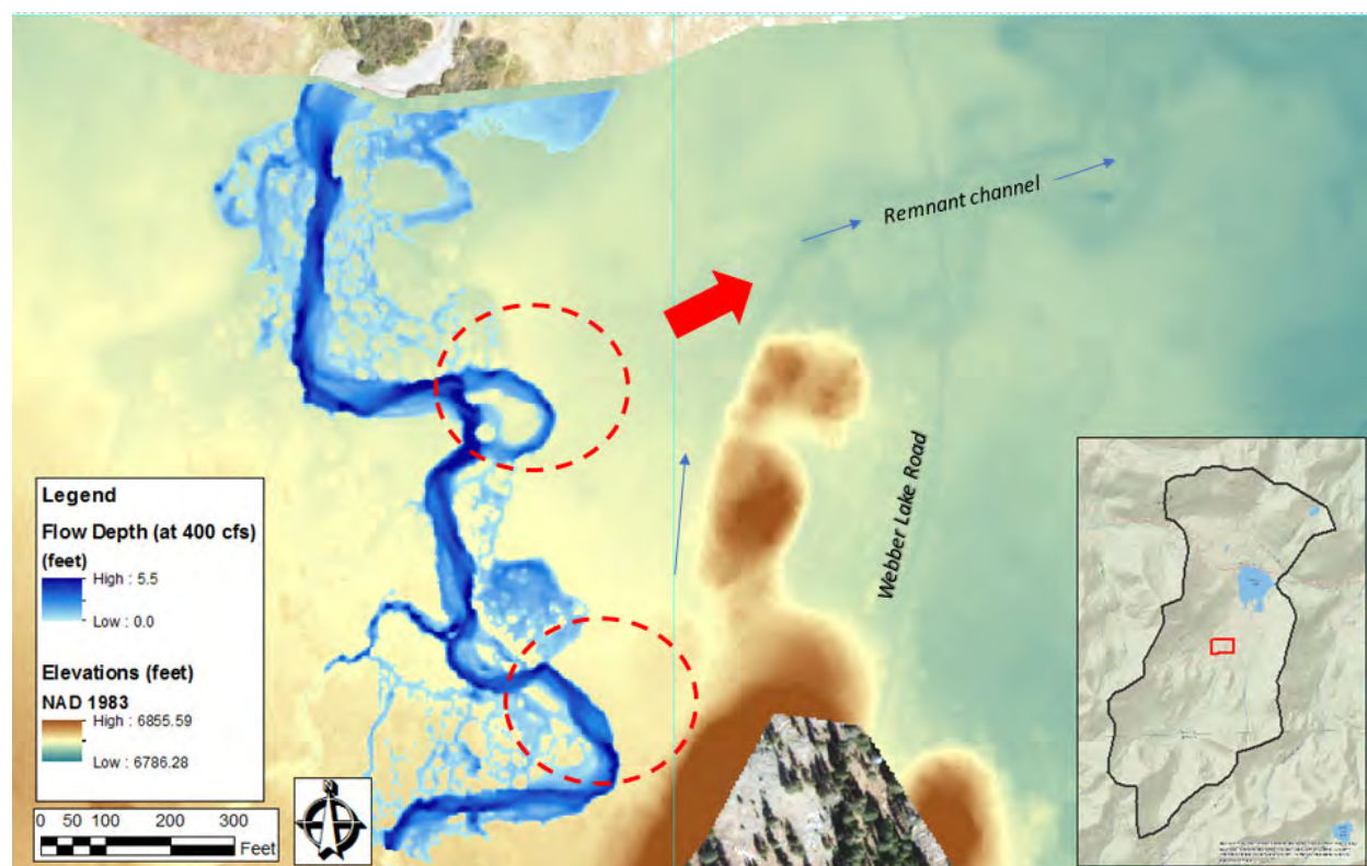
Figure 4-6 Hydraulic Model Results for WY2017 Peak Flow (estimated 400 cfs) in Existing Channel, Lower Lacey Meadow. Red arrow indicates remnant channel, while dashed circle identifies area proposed for splitting channel flow; flow direction is from bottom to top of page.
