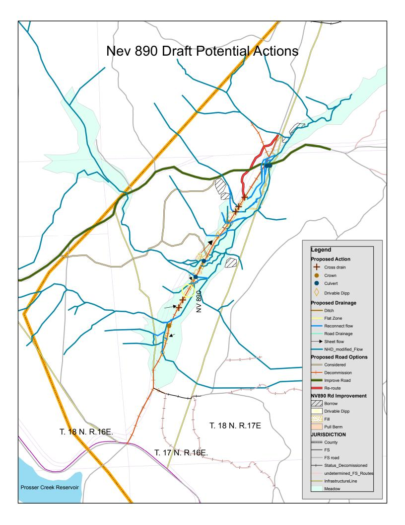
Proposed Design features are based on field visits and LiDAR. True field fit needs verification.
