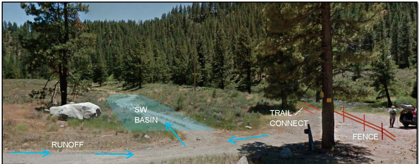
Figure 14. Illustration of maintaining drainage to stormwater basin and restoring northwest corner of project area.
