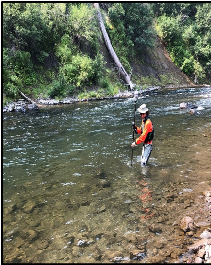
Figure 9. Collecting additional bathymetric data in deep water areas August 12, 2021.
