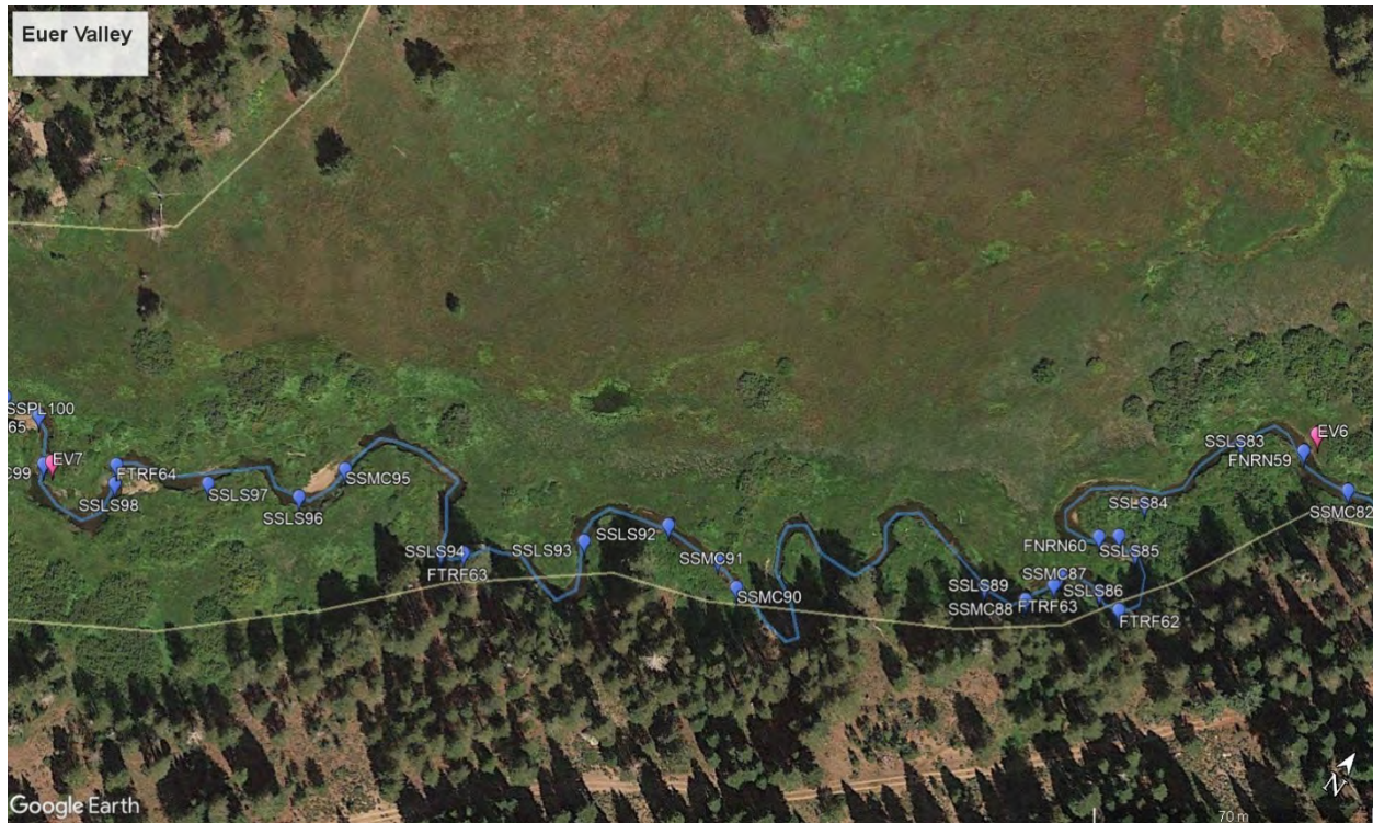
Figure 7. Reach EV6. The valley bottom is wider in this section but the stream channel is pinned tight to the moraine along the right meadow margin. This may have been intentionally diverted or channelized as livestock grazing impacts compounded. Historic channels are still present on the floodplain and likely still convey water in peak flows. Willows sprouted from a historic beaver dam are obvious adjacent to SSMC91.
