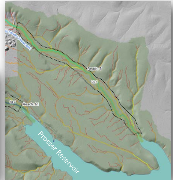
Flow accumulation analysis showing Reach T
