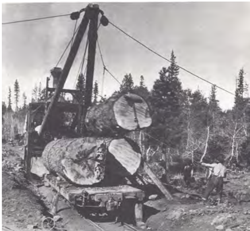
Photo 10. The McGiffert loader greatly speeded up log loading onto rail cars (courtesy Nevada Historical Society In Wilson 1992:13)
