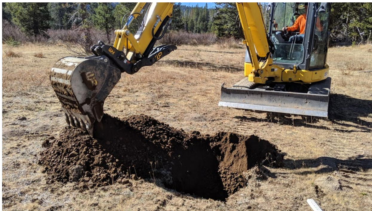
Figure 4-2 Soil Pit Excavated in a Remnant Channel, Upper Lacey Meadow. Note the occurrence of gravels 1.5 feet below surface.
