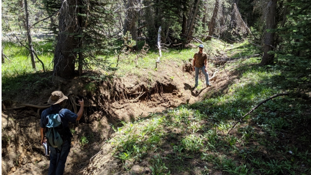
Figure 3-3 Example of Road Runoff Concentrated in a Natural Channel, Upper Lacey Meadow, Reach I (a).
