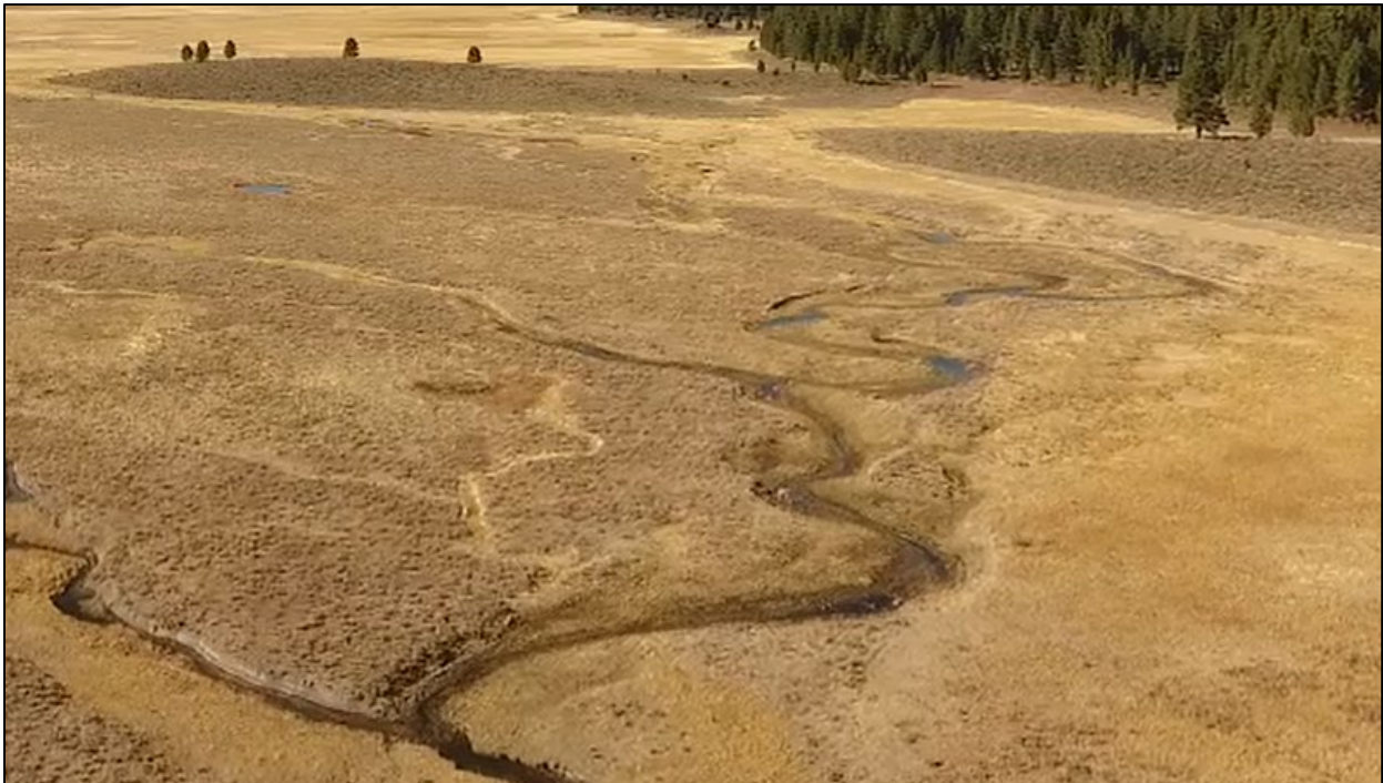
Figure 8. Upper Meadow at the northern end of project, looking upstream (west) at a spring-supported perennial swale system. Alternative A includes several earthen plugs to increase the depth, extent, and duration of ponded water in the channel and inset floodplain. Alternative B includes excavation of inset floodplains from adjacent upland areas to expand the extent of spring-fed perennial wet meadow across a greater area.
