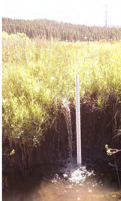
Reach 2 – Near confluence of Middle Martis Creek and Martis Creek. Lowered base level on Martis Creek, increased runoff, and focusing of drainage have led to headcut development and propagation. (photo credit: Brian Hastings, Balance Hydrologics)
