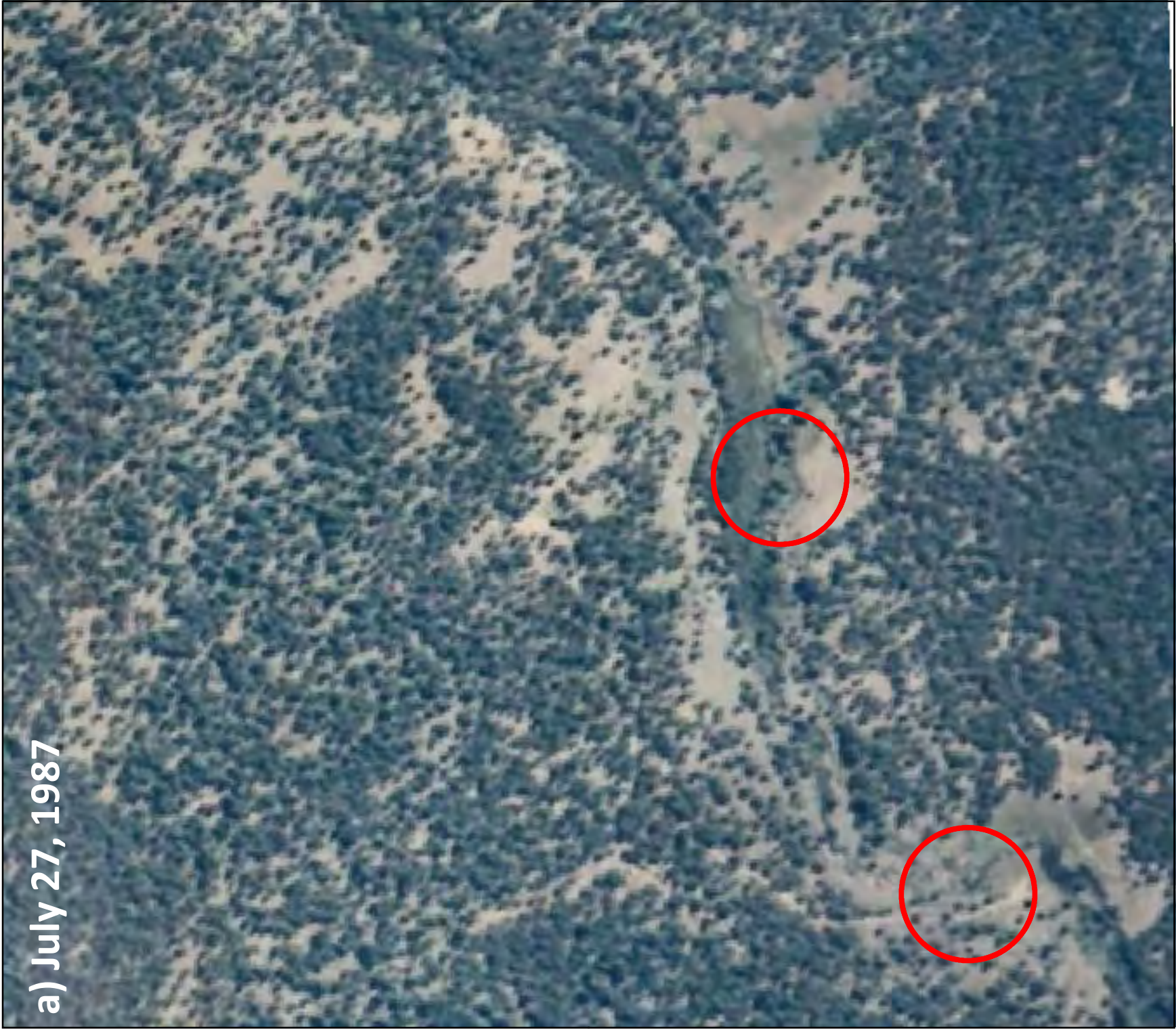
Figure 20. Selected changes in channel morphology: Martis Creek at Old Schaeffer Mill, Martis Valley; a) 1987; b) 1997. Red circles indicate visible erosion and deposition of sediment which may be the result of the January 1, 1997 flood. Historical disturbances (mill) may exacerbate the effects of floods.
