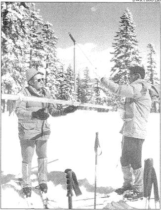
Department of Water Resources snow surveyors measure the water content of the snowpack. This information is used in forecasting spring runoff.
