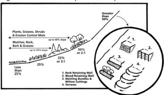
An inexpensive handheld inclinometer or a protractor can be used to determine the degree of slope in your project area and help you develop the most effective treatment for erosion control.
